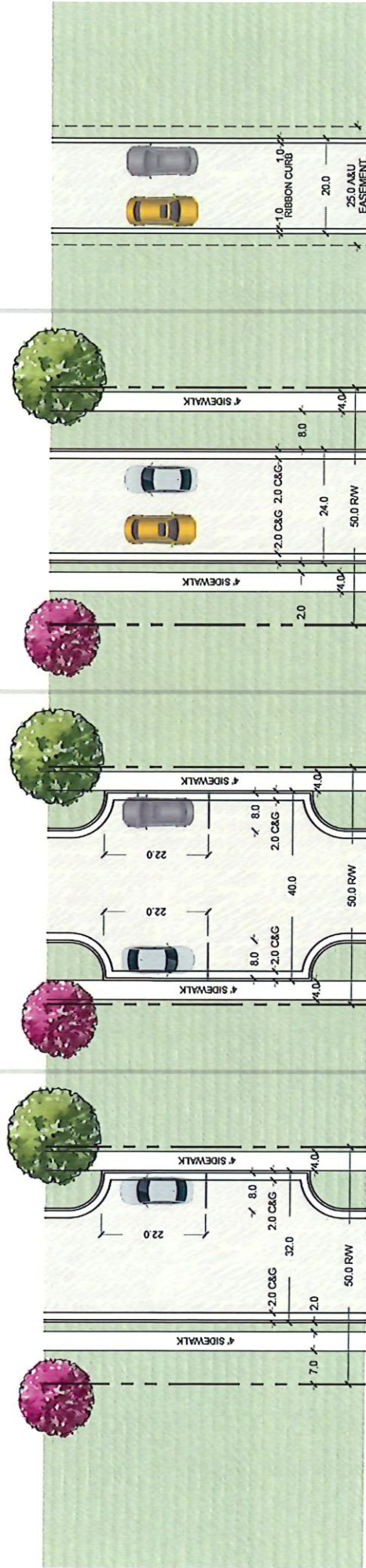
TYPICAL STREET PLAN TYPE #1 FOR ON-STREET PARKING (ONE SIDE)
